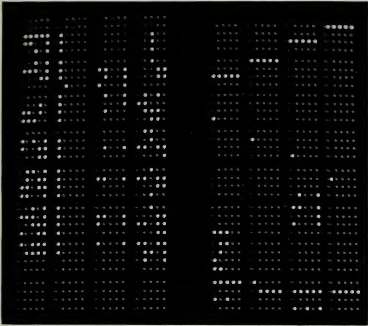
PLATE VI. A TYPICAL STORED PATTERN ON A CATHODE- RAY-TUBE SCREEN
